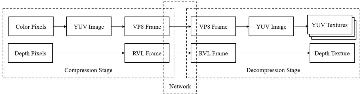
Figure 1. Overview of compression and decompression of our system. The compression stage is for the laptop connected to a Kinect v2. After the compression, the VP8 frame and the RVL frame get transmitted to a HoloLens. The decompression stage is for the HoloLens that received the frames.
